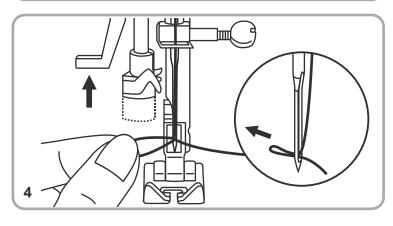
4. Hold the thread loosely and release the lever slowly. The hook will turn and pass the thread through the eye of the needle, forming a loop. Pull the thread through the eye of the needle.
