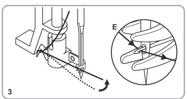
Take the thread in front of the needle and make sure it is under the hook pin (E). Then hold the thread slightly upwards so that it hangs on the hook.
