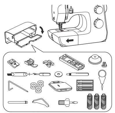
If you want to sew on the arm bed, pull out the snap-in sewing table (7) in the direction of the arrow.
