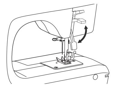
When sewing thick fabrics, the passage of fabrics under the presser foot (9) can be improved by raising the two-step presser foot lifter (18) further (arrow).
