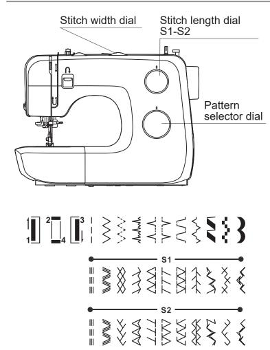
For **straight stitch**, turn the pattern selector dial (6) until the straight stitch coincides with the mark. You can adjust the needle position from central to right by turning the stitch width dial from "0" to "5".
