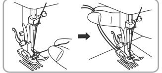
Pull on the upper thread to bring the lower thread up through the stitch plate hole. Lay both threads to the back under the presser foot (9).
