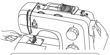
Hold the end of the upper thread with the left hand. Turn the handwheel (21) in the anticlockwise direction until the needle is again raised (a complete revolution).
